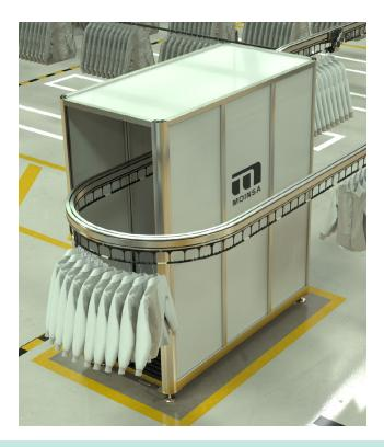
Fast, automatic, and error-free identification of garments on hangers. The information captured from each RFID tag is sent in real time to the management software, facilitating processes such as inbound control, classification, traceability, and dispatch, all without manual intervention.
